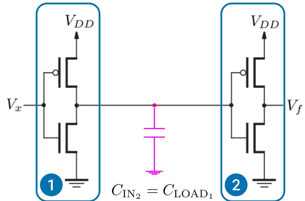
\*The *higher* the load capacitance, the *slower* the gate whose output is connected to it
