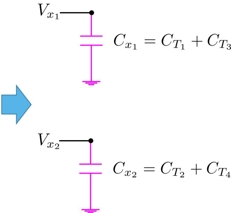
Input gate capacitance of the NOT gate acts as the **load capacitance** for the preceding NAND gate
