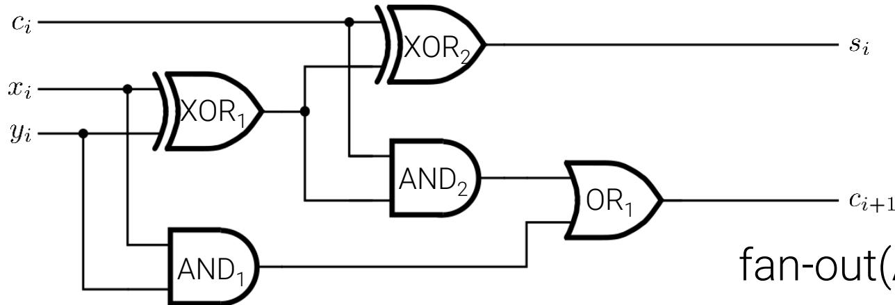
fan-out(AND<sub>1</sub>) = fan-out(AND<sub>2</sub>) = 1
