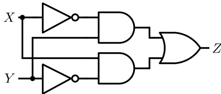
$$Z = \overline{X} Y + X \overline{Y} = X \oplus Y$$
