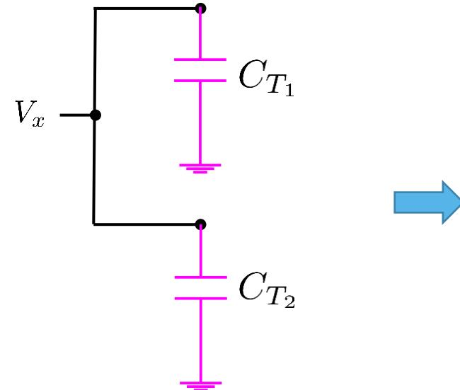
**Equivalent capacitance** of two or more capacitors connected **in parallel** is the **sum** of their individual capacitances
